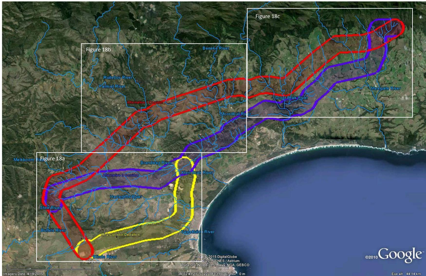
Figure 17: Overview of Freshwater constraints map in Google Earth showing the alternative routes for the proposed new power line, where the red line represents Alternative 1, the purple line Alternative 2; the yellow line the Deviation of Alternative 2 and blue lines indicate rivers
