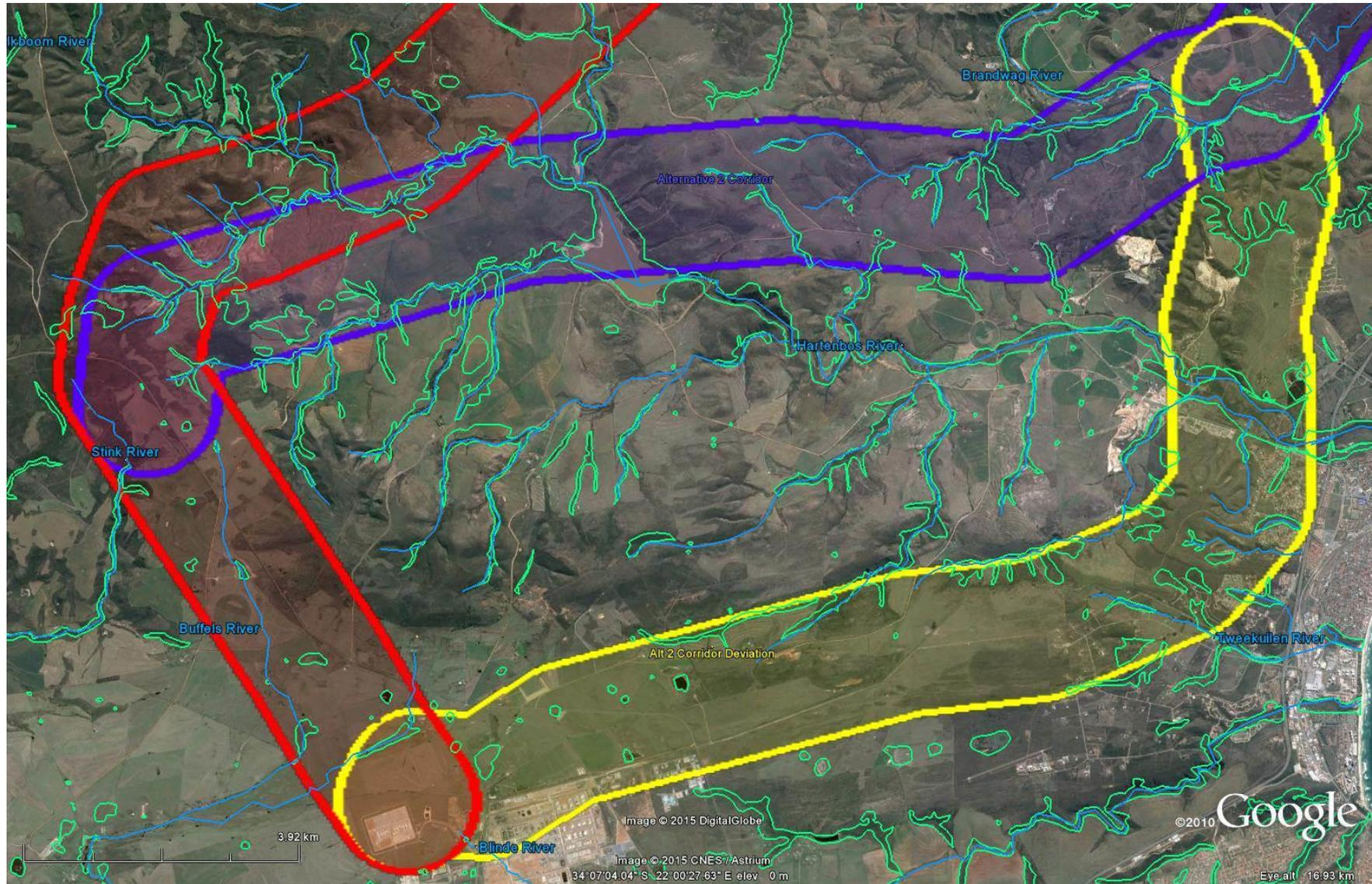
Figure 18a: Freshwater constraints map (Part 1) in Google Earth showing the alternative routes for the proposed new power line, where the red line represents Alternative 1, the purple line Alternative 2 and the yellow line the Deviation of Alternative 2; blue lines indicate rivers and green polygons wetland areas
