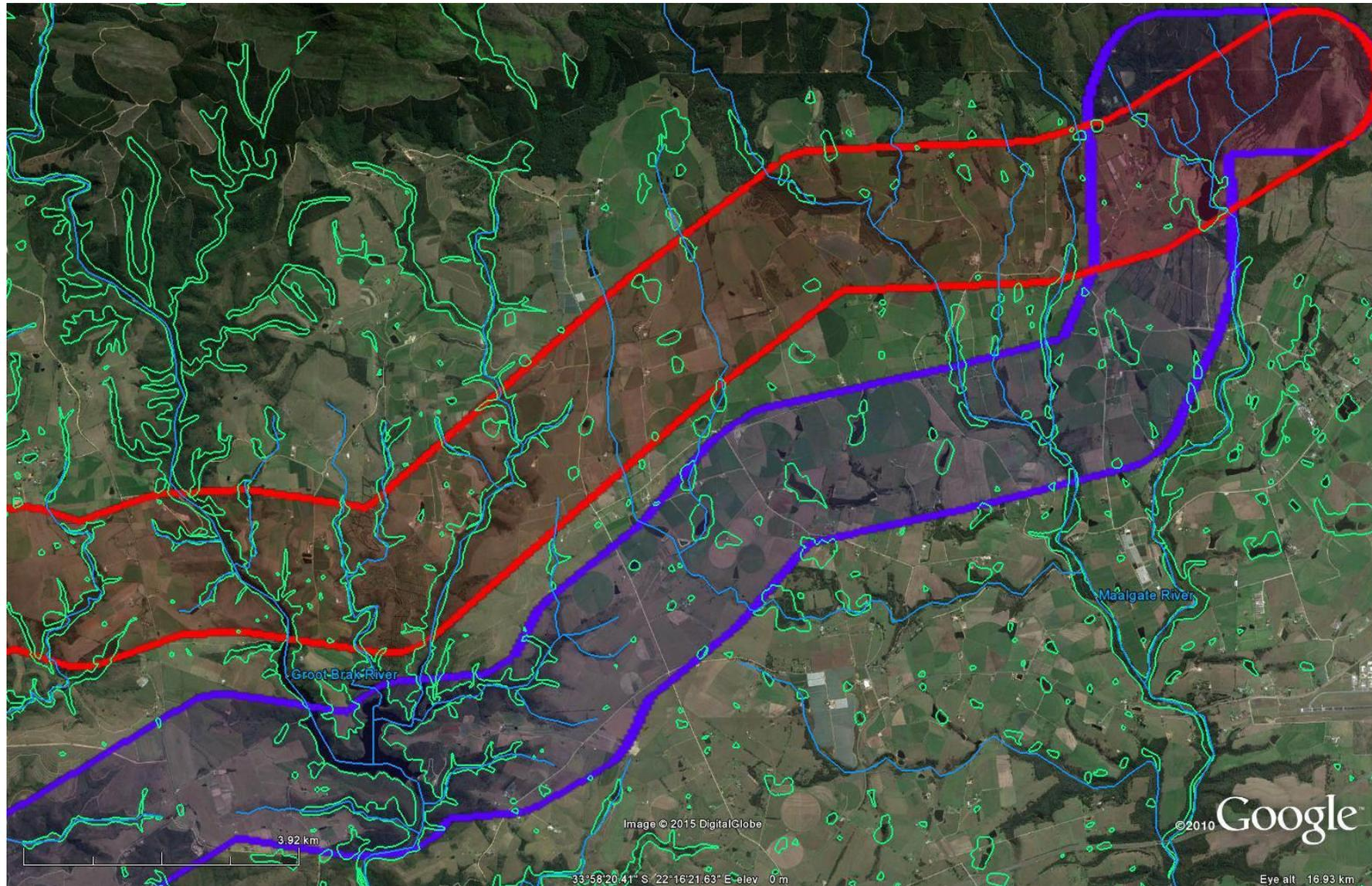
Figure 18c: Freshwater constraints map (Part 1) in Google Earth showing the alternative routes for the proposed new power line, where the red line represents Alternative 1, the purple line Alternative 2; blue lines indicate rivers and green polygons wetland areas
