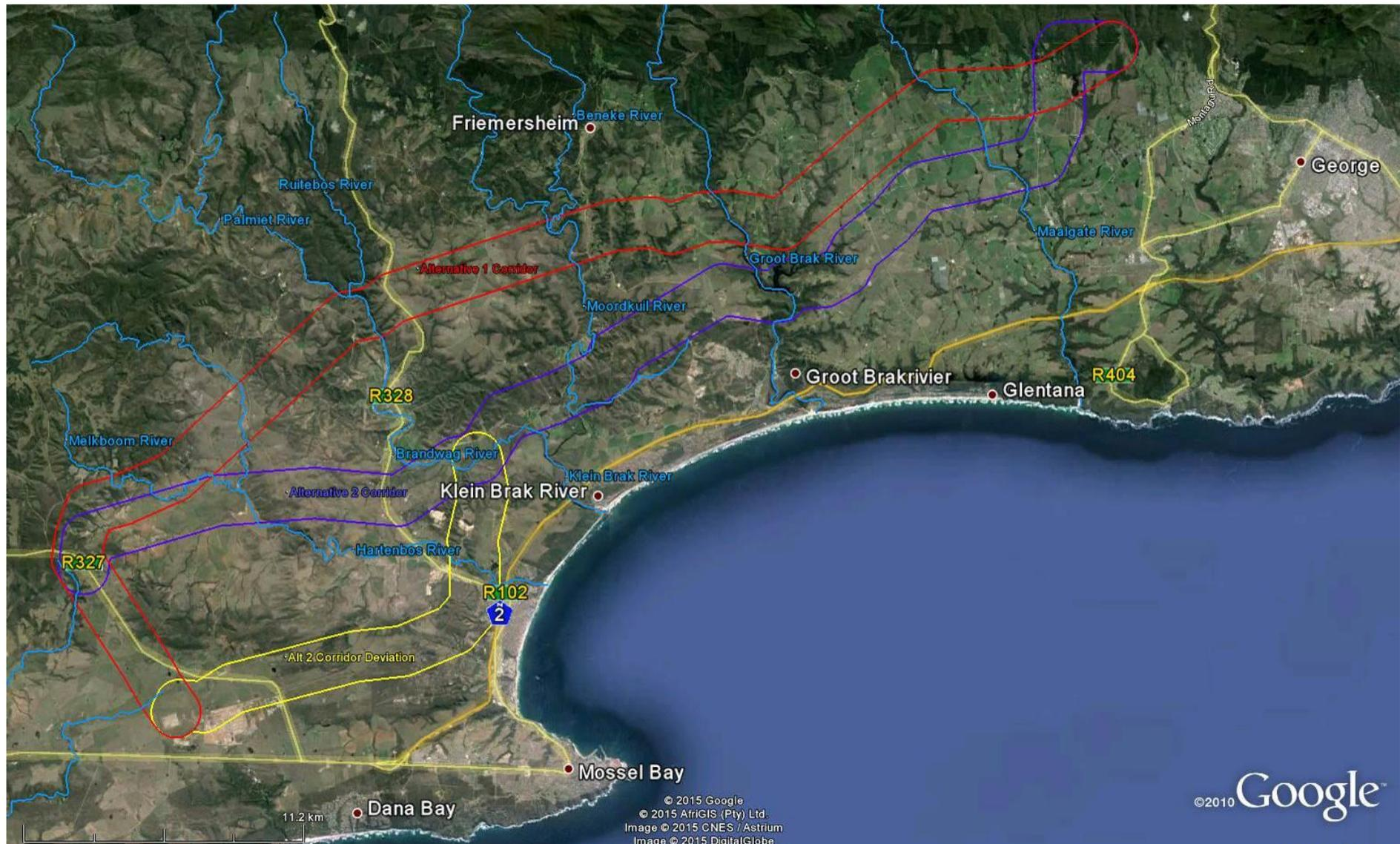
Figure 2: Google Earth image showing the alternative routes under consideration for the transmission line between Gourikwa and Blanco
